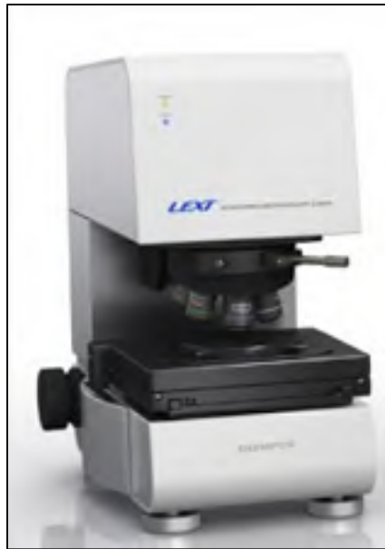
Figure 2.20 Microscope optique LEXT OLS4100 (Olympus)
