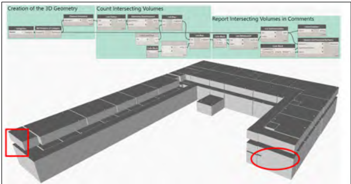
Figure 3.3 Dynamo script for Room/Space visual inspection
