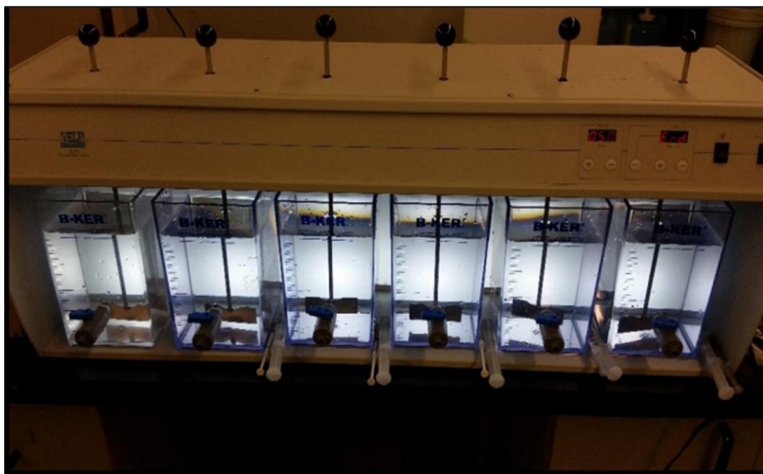
Figure 2.5 Banc de coagulation-floculation en b chers
