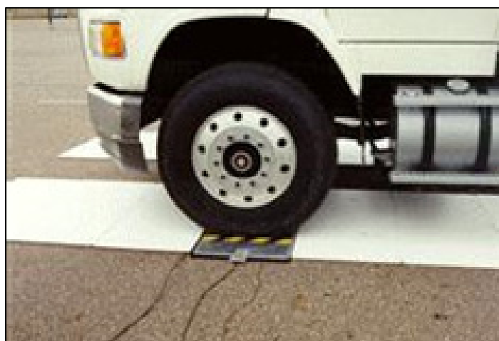
Figure 3.20 Tapis Capacitifs (Sun et al., 1998)
