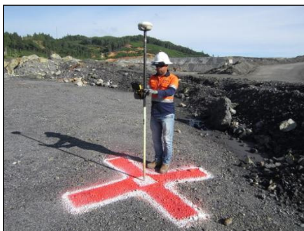
Figure 2.8 Marquage de GCP ( https://support.dronedeploy.com/docs/working-gcp-step-by-step )
