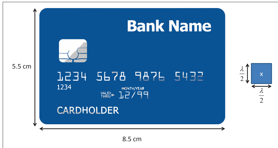
Figure 1.2 Example of compactness of millimeter-wave antenna elements. At a carrier frequency of f_c = 30 GHz (i.e., \lambda = 1 cm), and with \lambda/2 antenna spacing, more than 180 antennas can be placed on an area as large as a credit card
