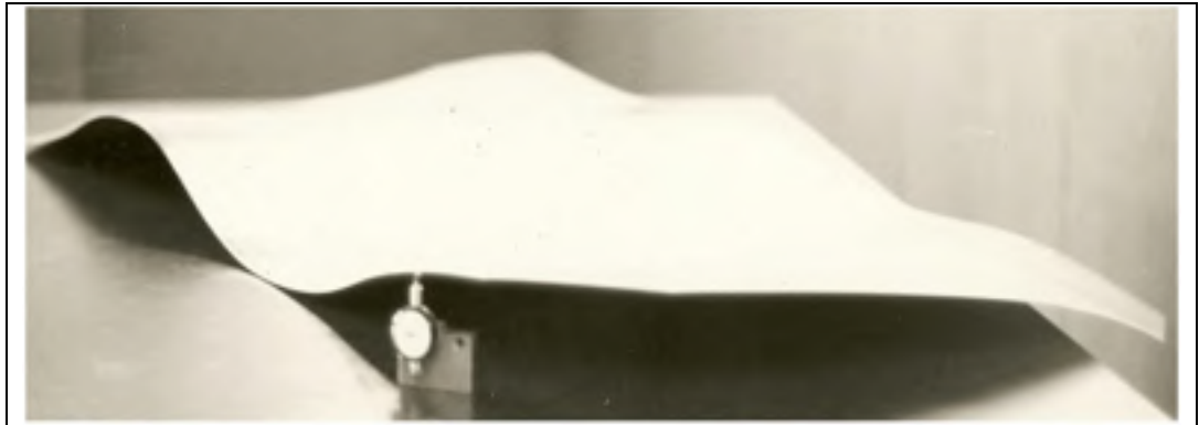
Figure 1-9 A distorted part after quenching process (CROUCHER, 2008)
