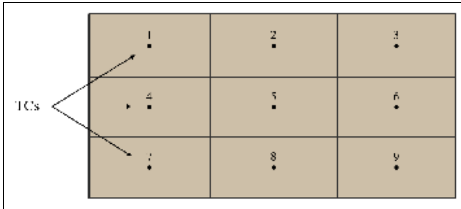
Figure 4-3 The subdivision of the part in 9 zones and the location of the thermocouples.
