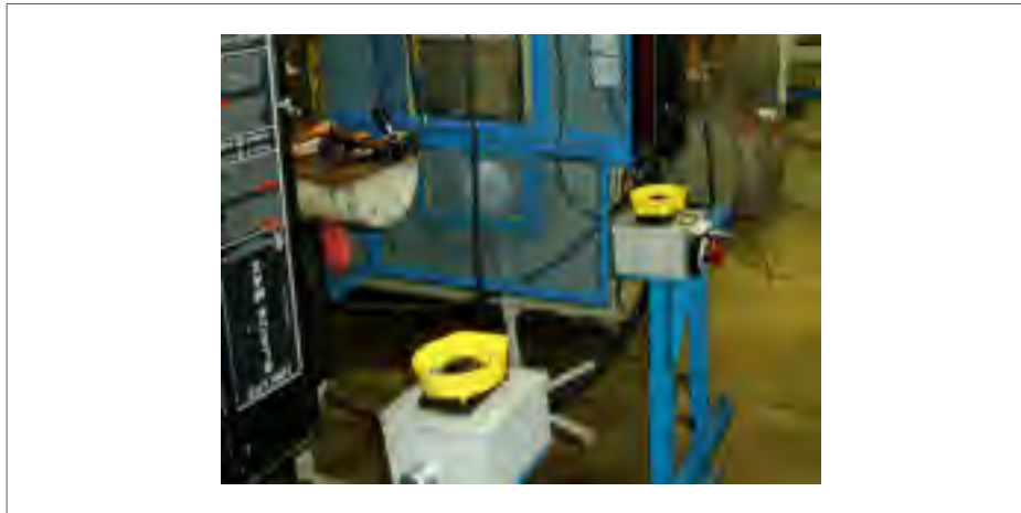
Figure 7.1 Mechanical punch press with redundant protective devices
