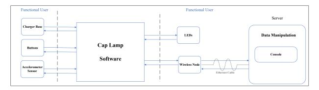
Figure 2.2. Context diagram of cap lamp software
