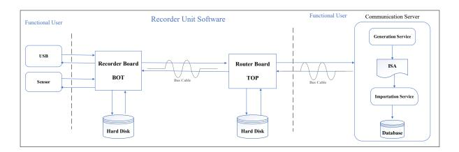
Figure 2.1. Context diagram of recorder unit software
