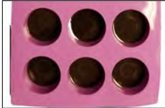
Figure 2.2 Silicone molding of BDS samples
