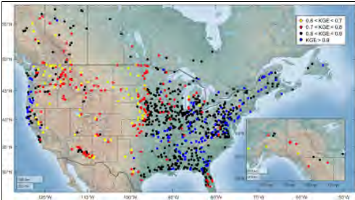
Figure 3.1 Location (centroid) of the 921 study catchments with their KGE calibration performance bracket: yellow (0.6 to 0.7); red (0.7 to 0.8); black (0.8 to 0.9) and blue (above 0.9)
