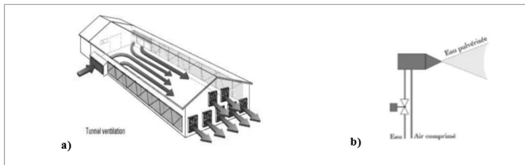
Figure 1-2 a. Ventilation tunnel, b. Buse de brumisation
