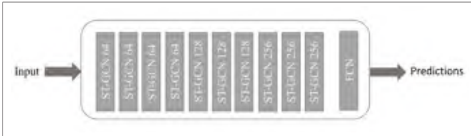
Figure 2.3 Spatial temporal graph convolution network architecture
