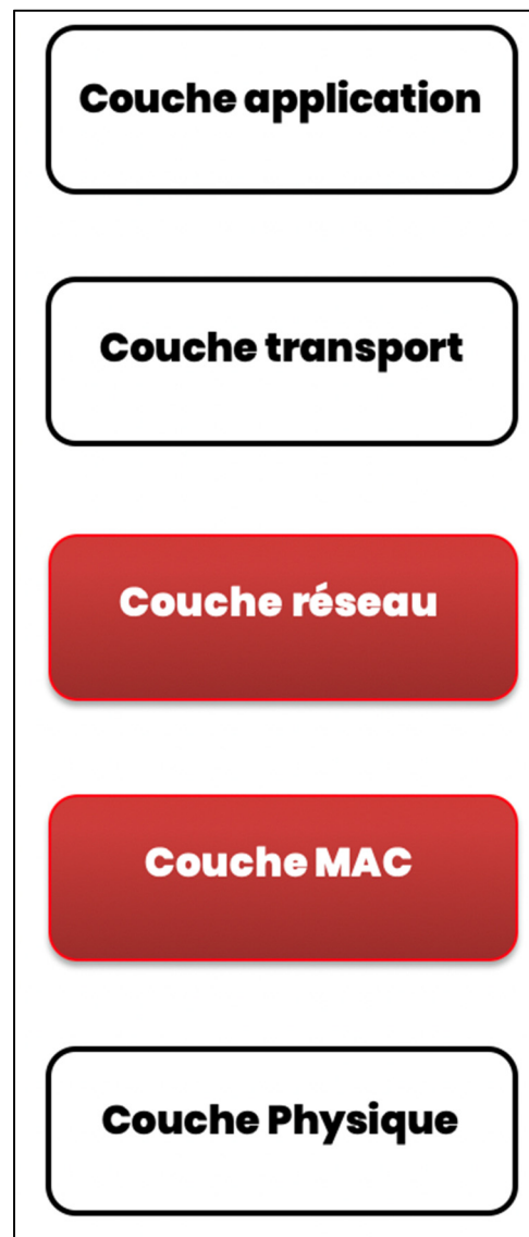
Figure 2.1 Pile de protocoles OSI
