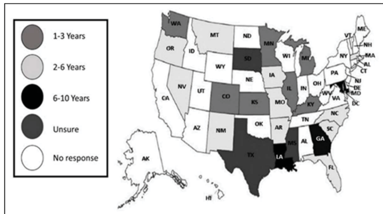
Figure 3.1 Mean service life of a 40-50 mm HMA overlay installed on a cracked pavement in the United States (adapted from (Kwon, et al., 2005))
