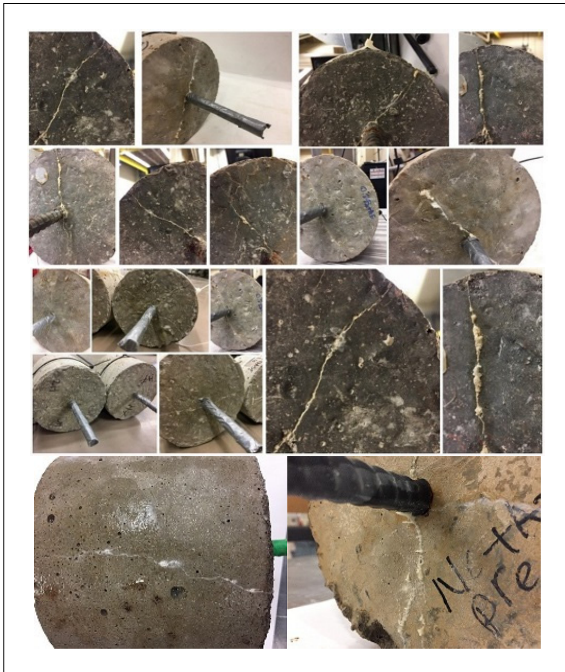
Figure 6.23 Healing products at the external crack surface of pull-out specimens of SAP-based NC mixtures with and without AE
