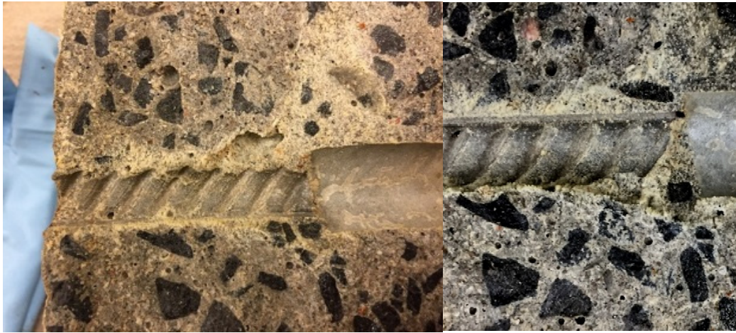
Figure 6.43 Healed products (white powder) content around the rebar as compared to the bulk matrix (AE concrete containing 0.25% SAP)
