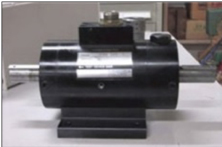
Figure 3.4 Torque transducer in the Gifu Simulator at the Human Support Systems Laboratory at Gifu University, Gifu, Japan (Bando et al., 2004)
