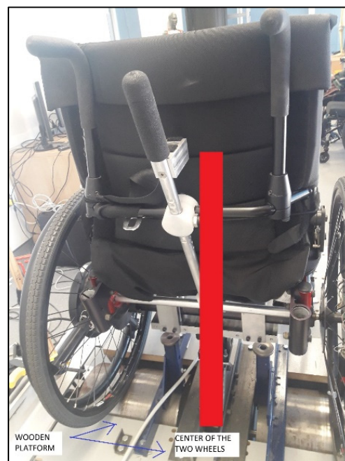
Figure 3.11 Force cell placement on the simulator platform
