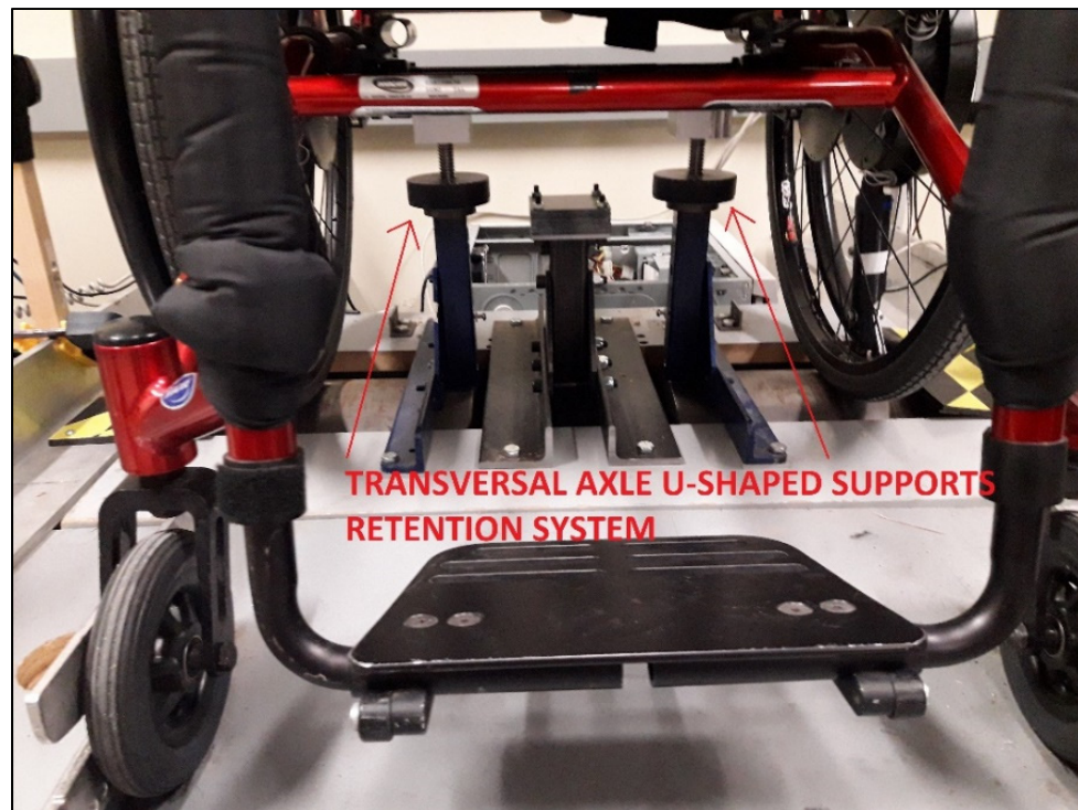
Figure 1.34 LIO Simulator retention system: transversal axle U-shaped supports
