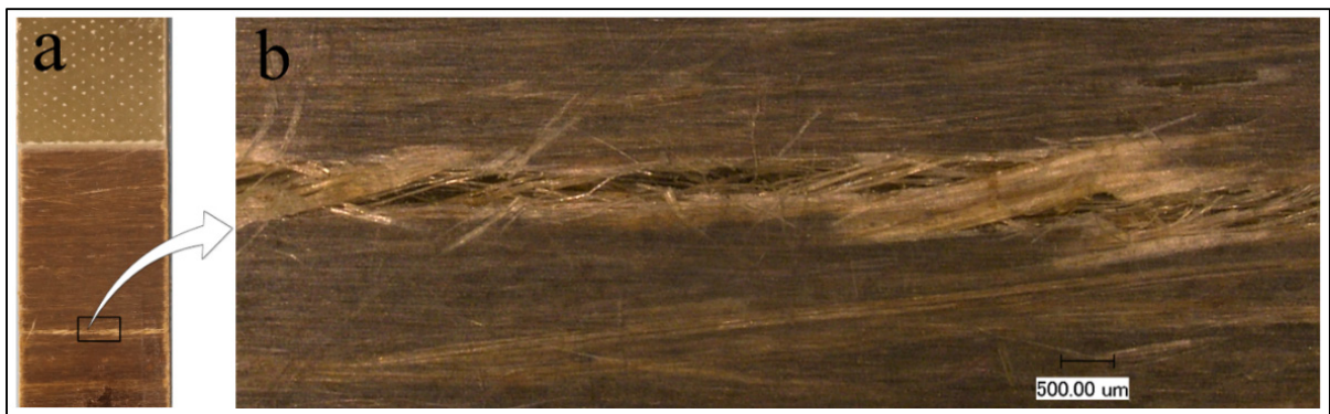
Figure 3.7 Failure modes in transverse tensile loading; fracture path (a) and failure mechanisms (b)
