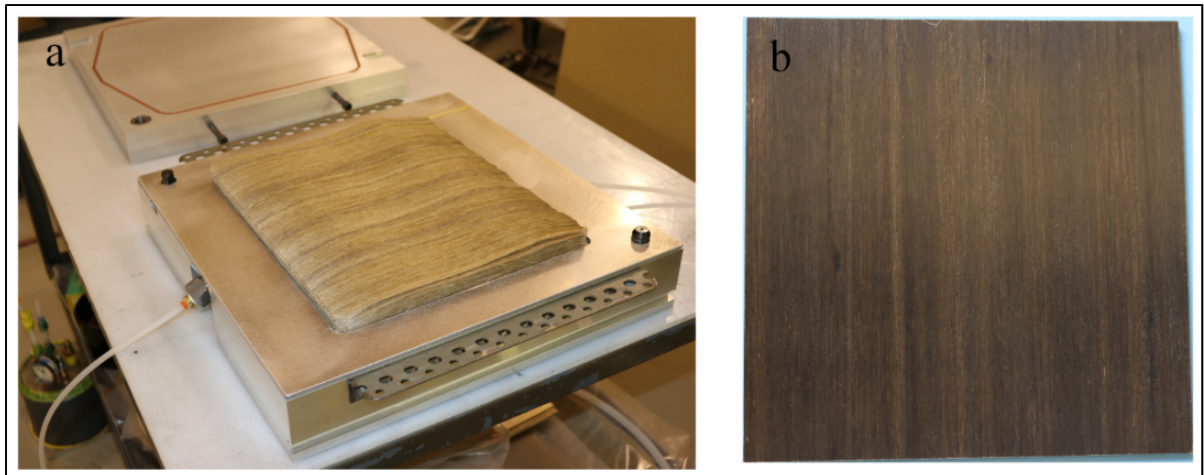
Figure 3.1 Mold and typical reinforcement stack used for RTM injection of composite laminates (a) and final UD flax-epoxy composite (b)
