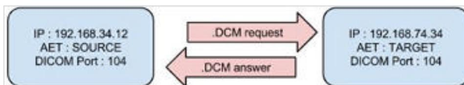
Figure 2.16 C-Find Transaction diagram
