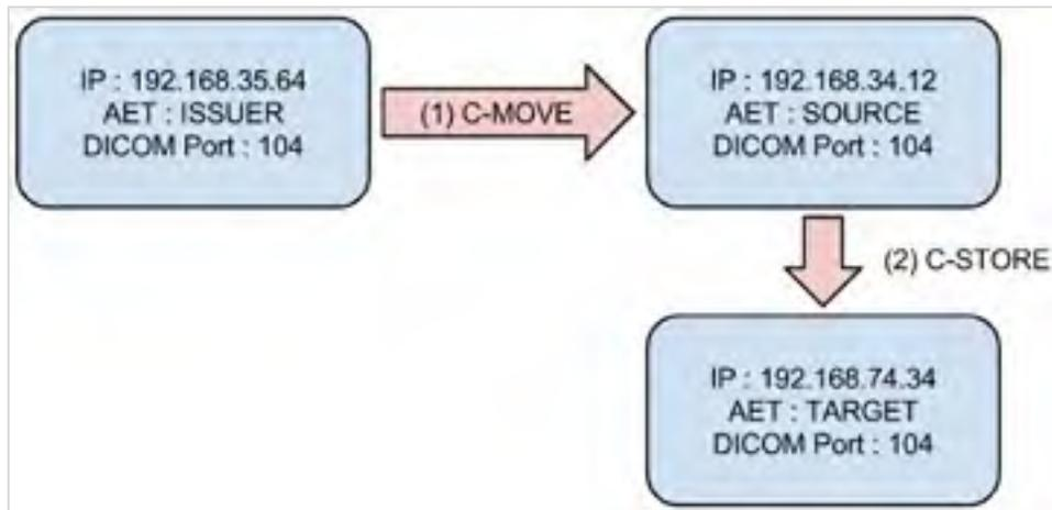
Figure 2.17 C-Move and C-Store transaction diagram
