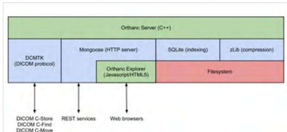
Figure 2.8 The layer of Orthanc server software architecture
