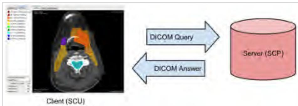
Figure 2.14 Transaction between Service Class User (SCU) and Service Class Provider (SCP)
