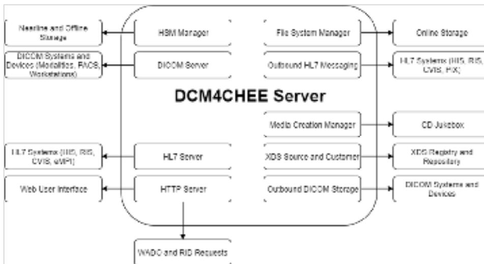
Figure 2.2 DCM4CHEE Server system architecture
