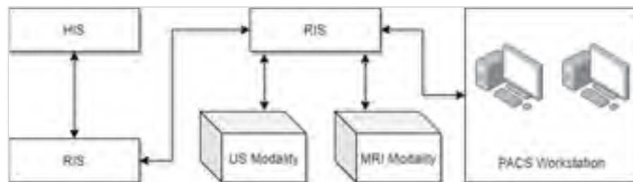
Figure 3.3 Typical connections of PACS in hospital systems
