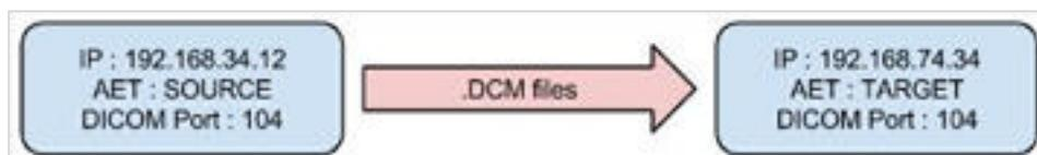
Figure 2.15 C-Store command transaction diagram
