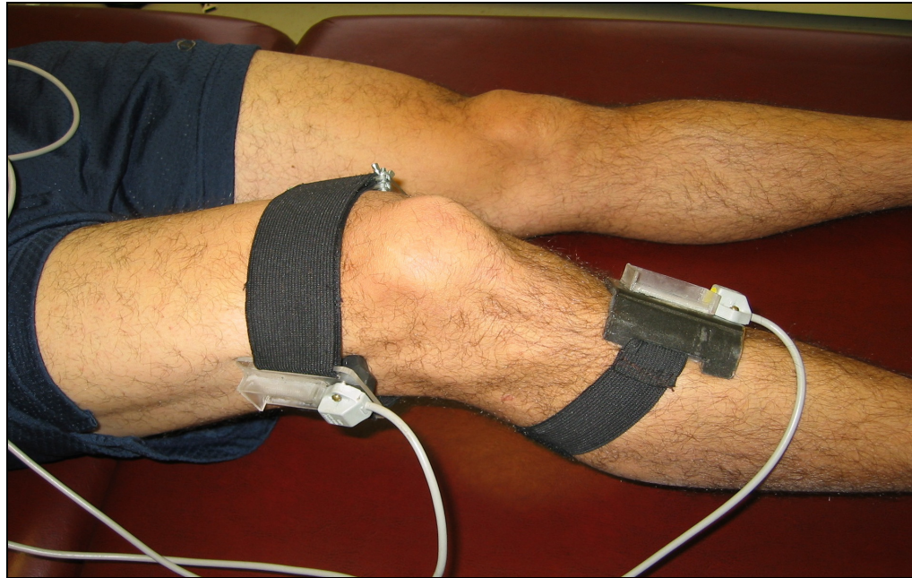
Figure 7.2: Electromagnetic motion capture device attached to a subject's lower limb using an attachment system developed with the objective of diminishing skin to bone movement artifacts.
