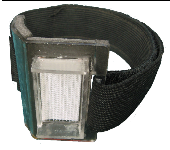
Figure 4.2 The tibial component of the attachment system we developed for data acquisition.
