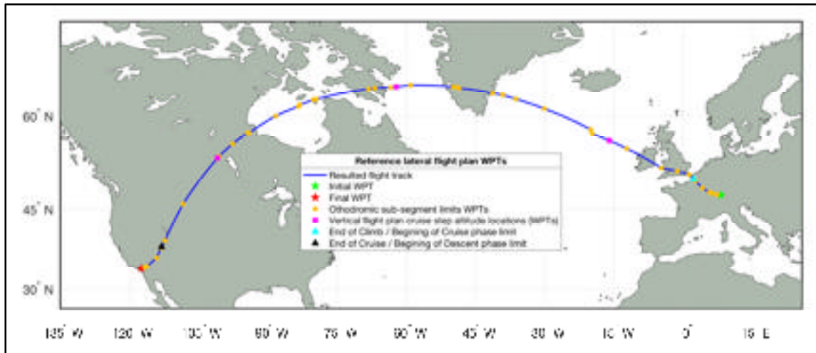
Figure 4.19 The significant WPTs of the reference lateral flight plan
