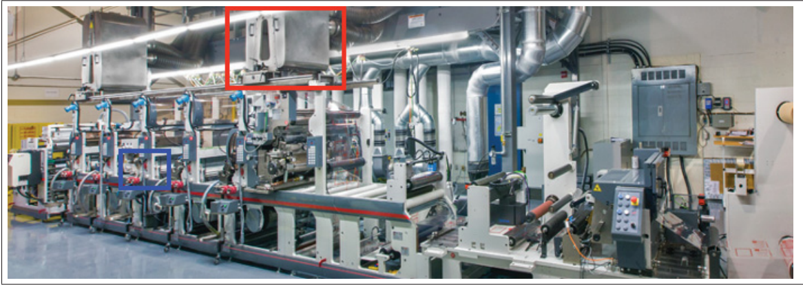
Figure 4.1 The industrial roll-to-roll printer consists of five printing units, where a blue rectangle indicates the location of the printing unit #3 used for the sample's fabrication. The red rectangle highlights the dryer module
