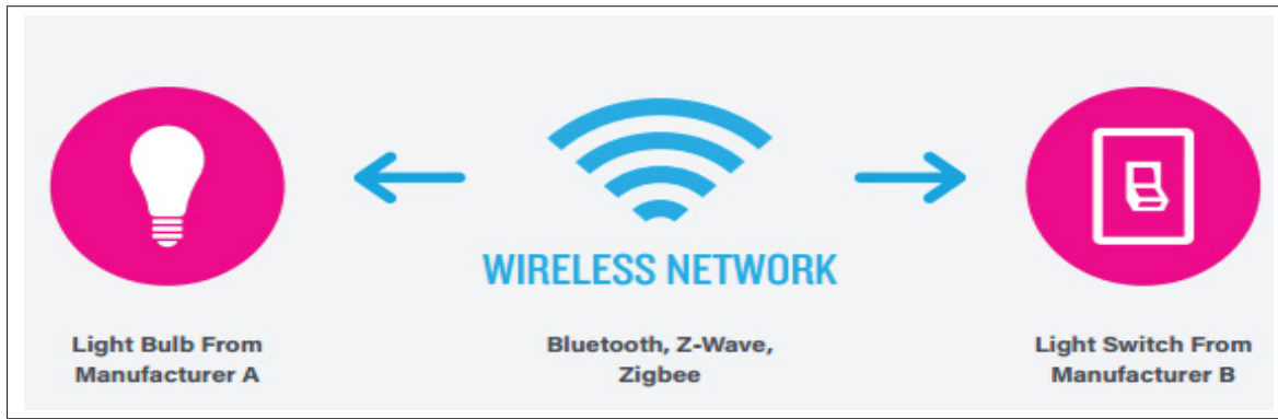
Figure 1.3 IoT Device to Device Communication Model Taken from Rose et al. (2015)
