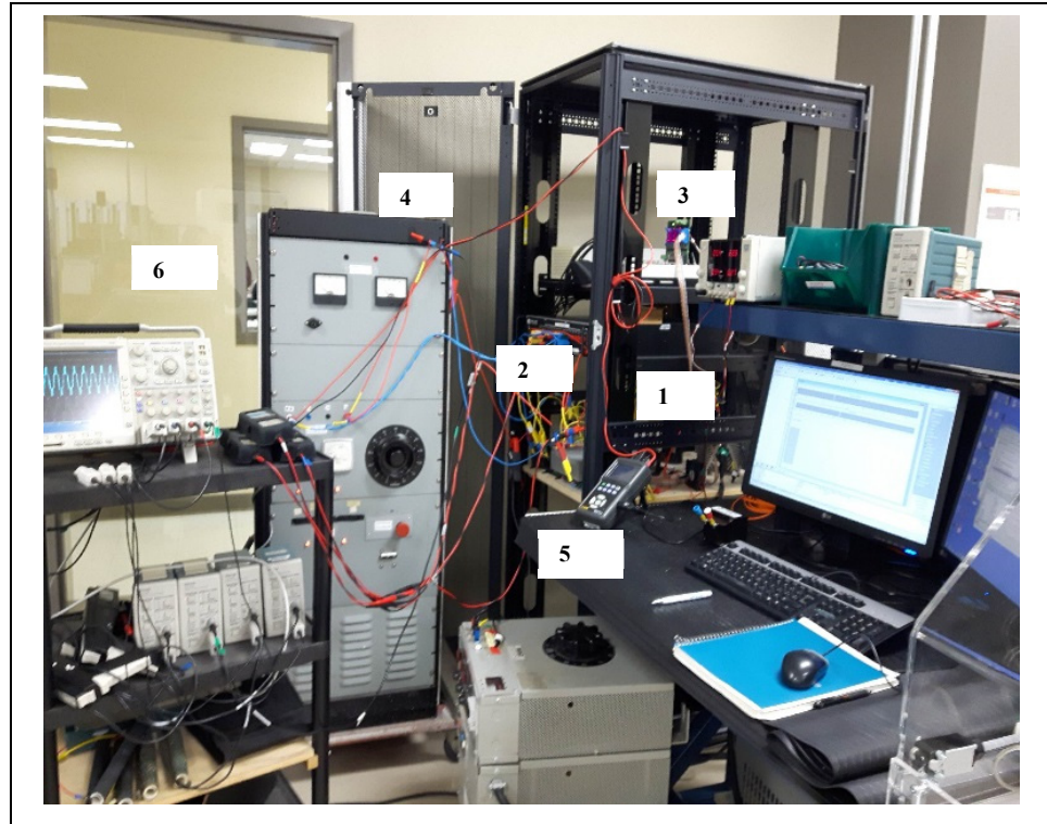
Figure 2.8 Experimental setup. (1) PUC5 inverter, (2) LCL filter, (3) dSPACE 1103, (4) grid, (5) DC source, (6) oscilloscope
