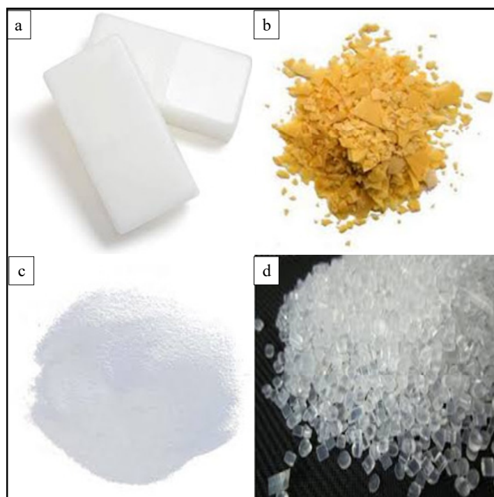
Figure 3-2 The appearance of the binders at room temperature a) paraffin wax, b) carnauba wax, c) stearic acid, and d) ethylene-vinyl acetate
