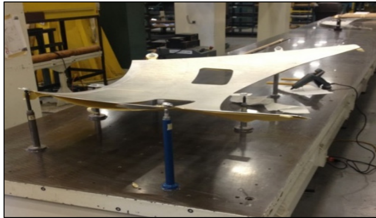
Figure-A I-1 Example of a specialized inspection fixture Bombardier Aerospace Inc.
