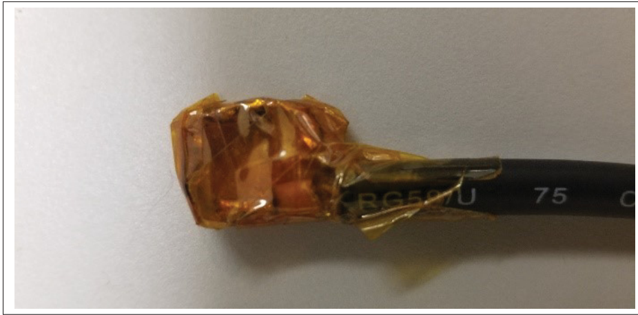
Figure 4.4 Magnetic field probe built from a coaxial cable covered with Kapton tape
