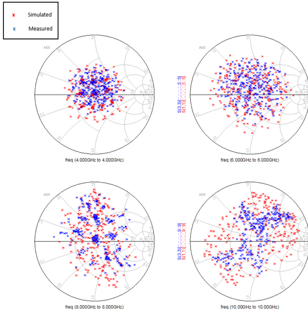
Figure 3.11 Simulated and measured S_{11} distributions for the 256 tuner states
