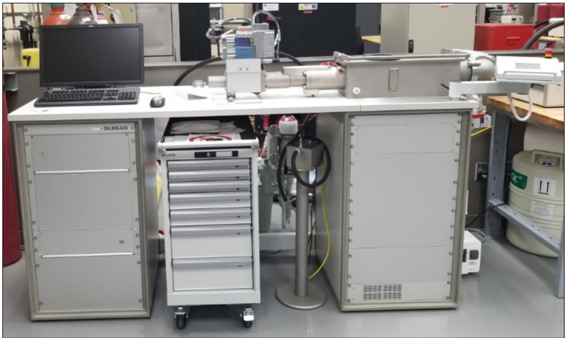
Figure 2-2 BAHR DIL805 high-resolution dilatometer Taken from BEN FREDJ Emna (2019)
