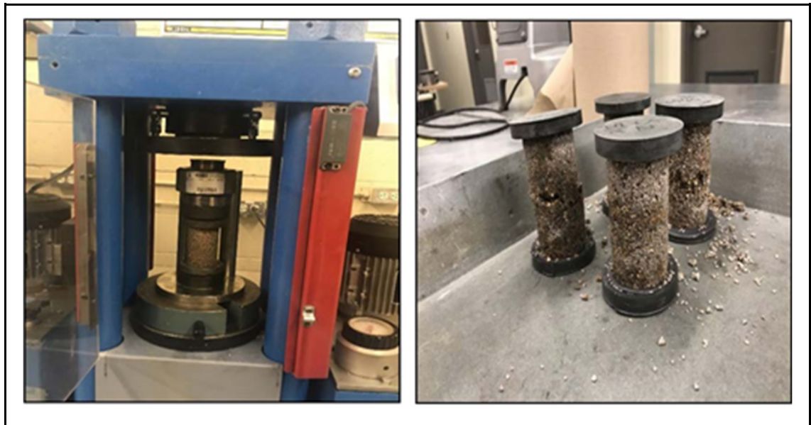
Figure 4.4 UCS apparatus (image on the left) and treated samples after failure (image on the right)
