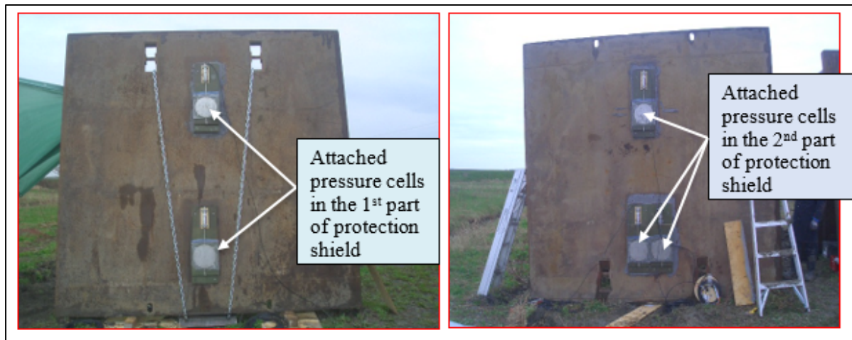
Figure 3.8 Pressure cells are fixed on the side of the first and second trench boxes
