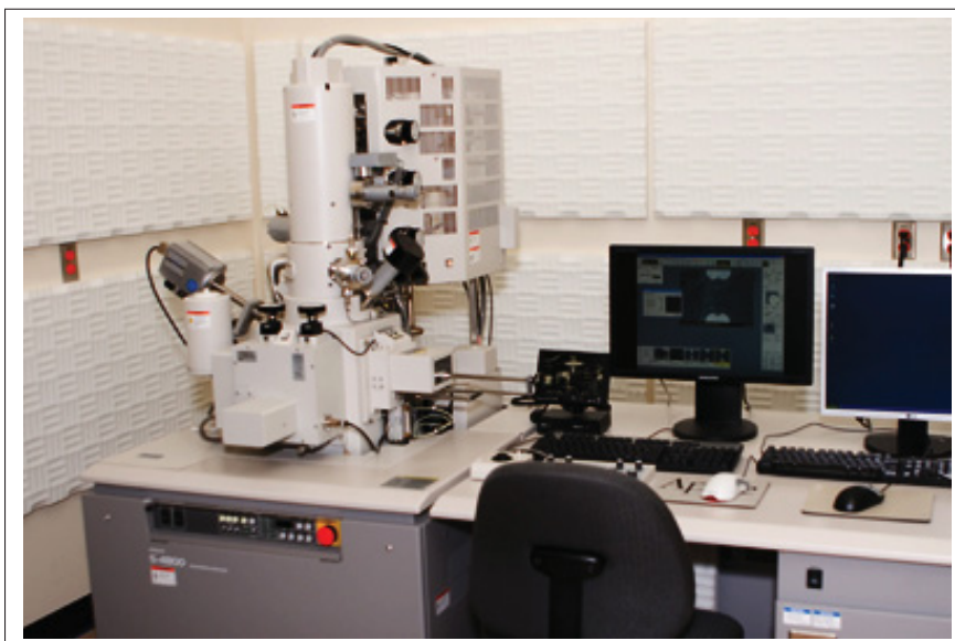
Figure 3.8 Scanning Electron Microscope (SEM, Hitachi S4800)
