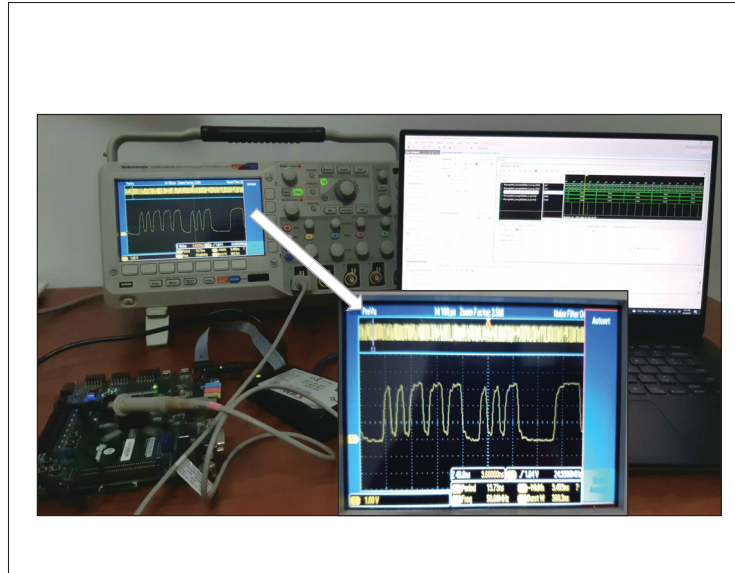
Figure 6.8 Hardware validation of the proposed PRNG. Only the LSB of the random data B_1 is observed in oscilloscope. The system is running at 50 MHz
