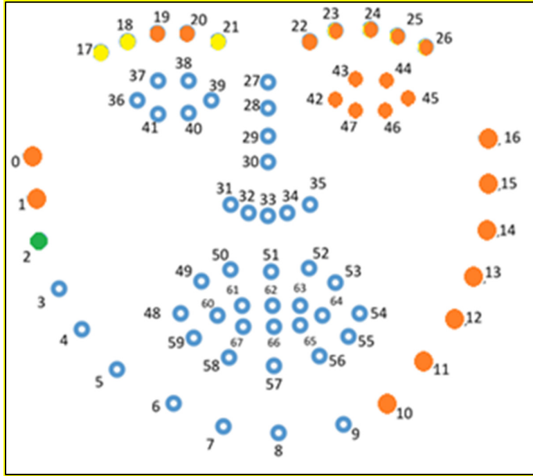
Figure 4.3 Face landmarks. The points shown are tracked on each frame of the videos. The points in yellow, green, and orange compose the best features in the automatic classification task. The yellow points are the points in 2D exclusively. The green point is the point in 3D exclusively. The orange points composed the best features in both 2D and 3D groups
