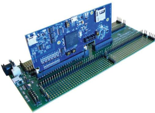
**Figure 1. TMDSDOCK28379D Experimenter's Kit**
