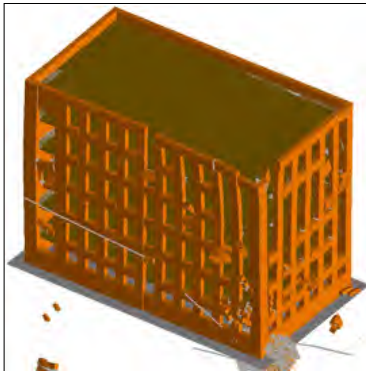
Figure 3.13 URMW building at Collapse Prevention level for Nahanni S3-EN1 ground motion record.
