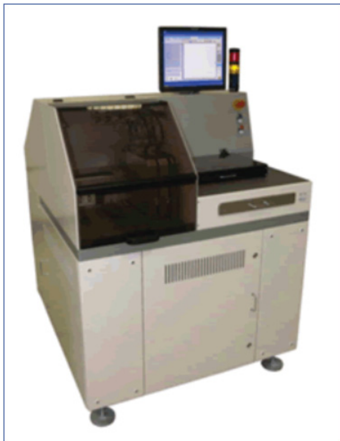
Figure 4.6 PAM4s punching machine
