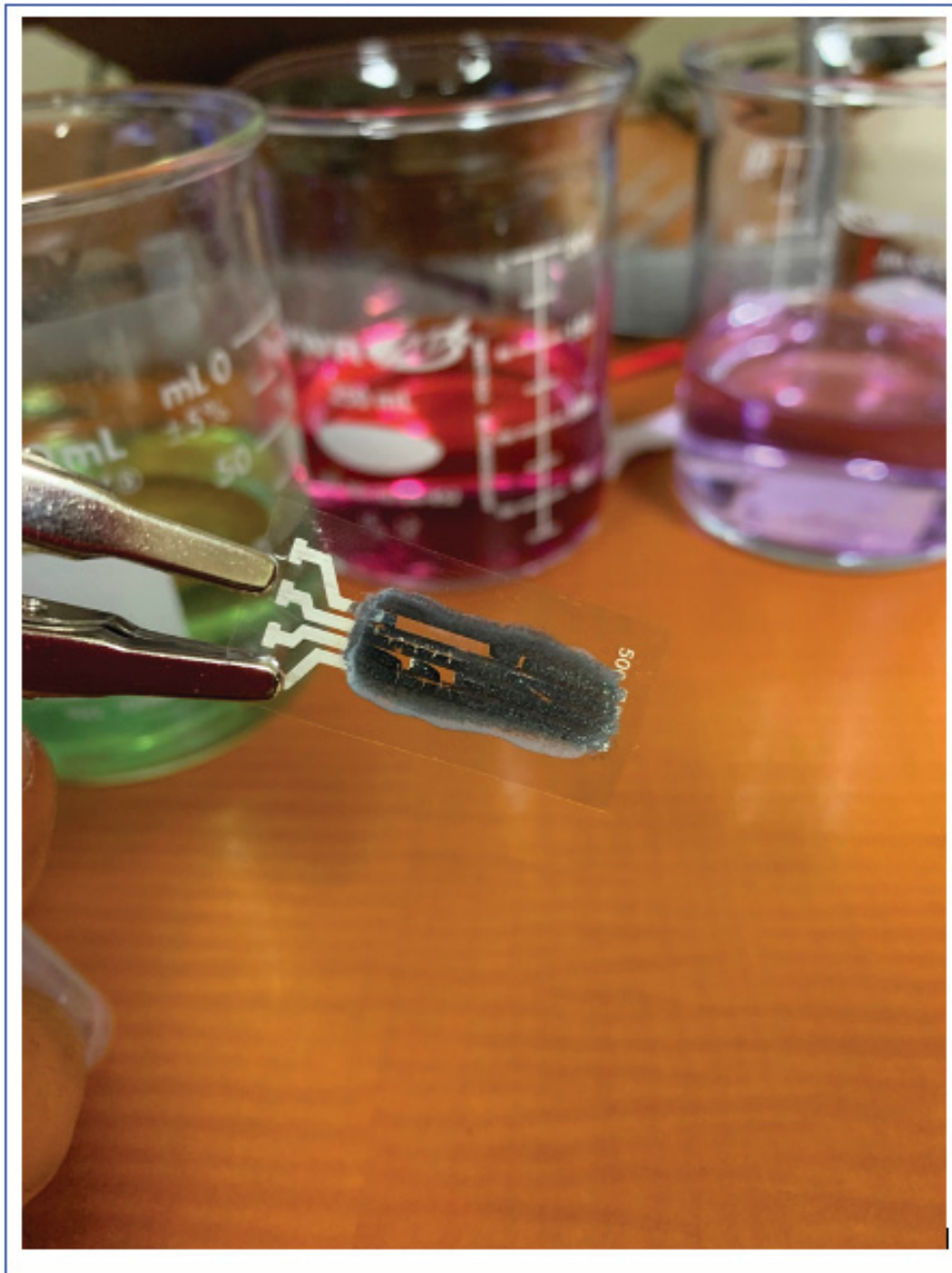
Figure 5.4 Broken composite film and silver electrodes on the substrate
