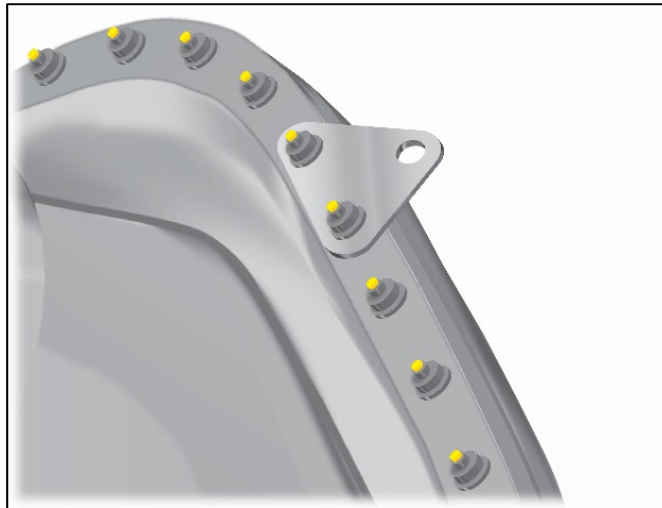
Figure 3.6 Bracket A secured to the structure in the final assembly location
