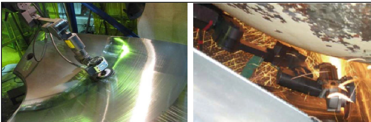
Figure 1.1 The SCOMPI robot in machining process Taken from Hazel et al. (2012b, p. 113)
