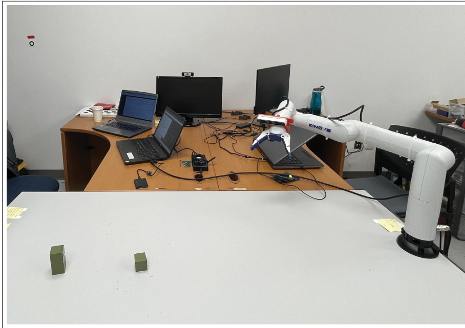
Figure 5.8 Alternative camera pose used for the 6 th scenario, resulting in a successful occlusion-free path-planning
