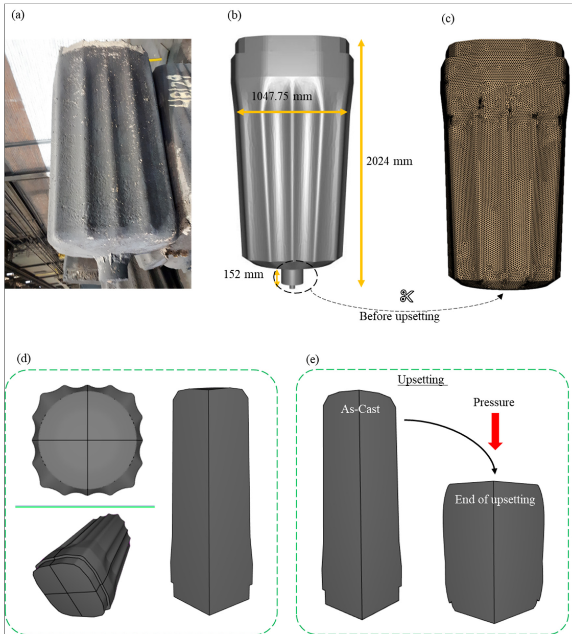
Figure 6.1 As-cast ingot (b) CAD model of ingot (c) Meshed model of 360° 3D (d) 90° of the model (one quarter) (e) Upsetting process
