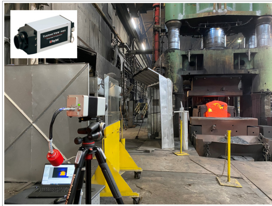
Figure 2.2 Forging temperature measurement by Thermal camera
