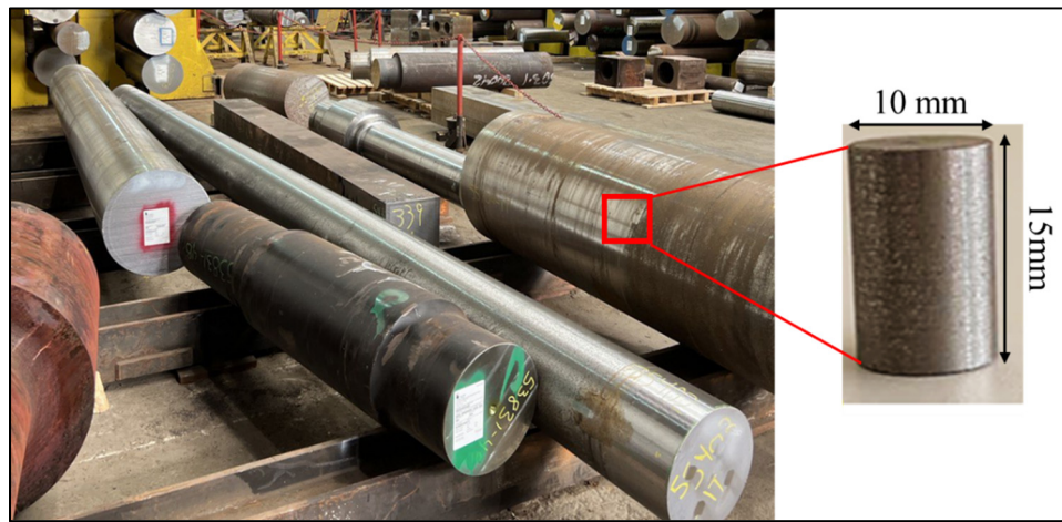
Figure 4.1 An image depicting the position of the Gleeble tests samples in the industrial-sized ingot
