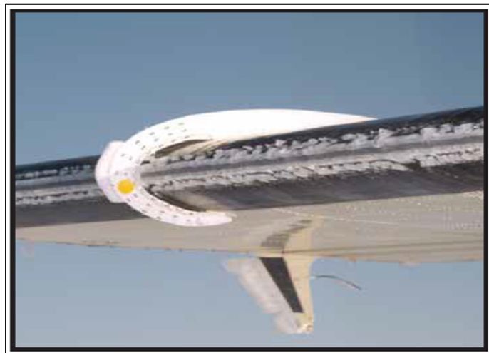
Figure 0-1 Ice formation on the wing's leading edge Taken from AOPA (2008)
