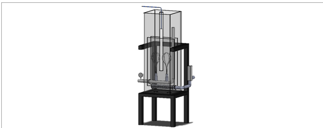
Figure 3.2 Handmade Submerged Membrane Photocatalytic Reactor (SMPR) taken from Ong et al. (2014, p. 50)
