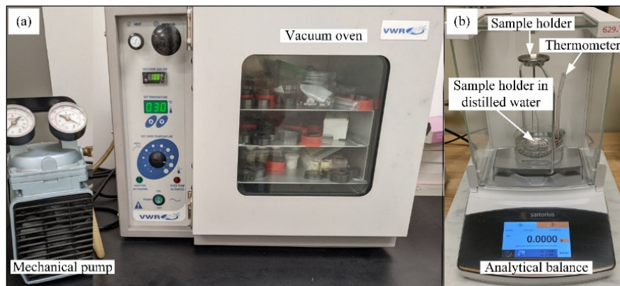
Figure 3.12 Sintered density measurement (a) vacuum oven and (b) Archimedes setup
