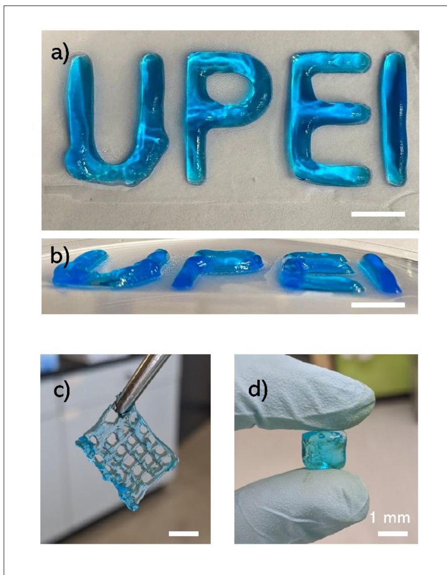
Figure 3.4 Various geometries printed using 3 wt% sodium alginate a) top and, b) side views of 4-layer UPEI letters, c) a 2-layer scaffold, and d) 3-layer cube. Reprinted with permission (Badr et al., 2022)
