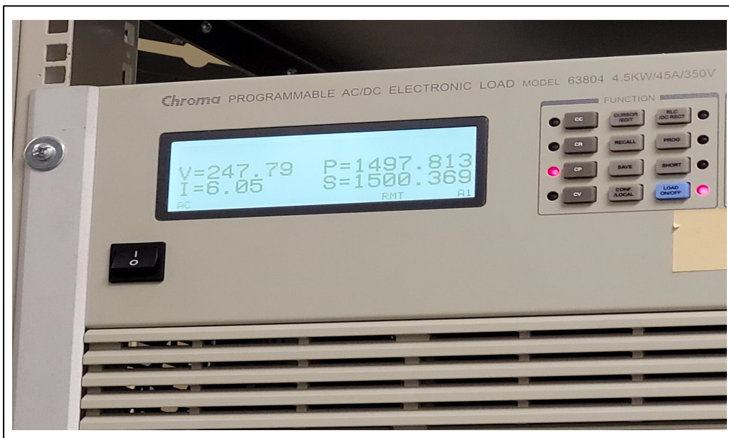
Figure 4.14 Chroma Load Pack Measurement via Control Panel
