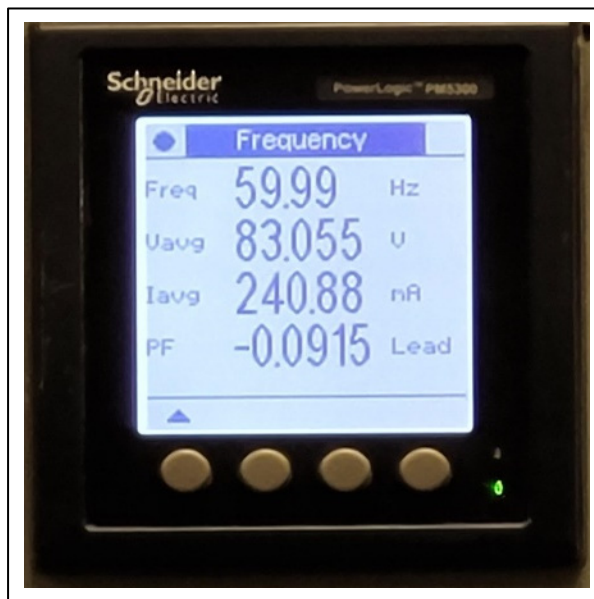
Figure 4.11 Grid Frequency Read from HMI
