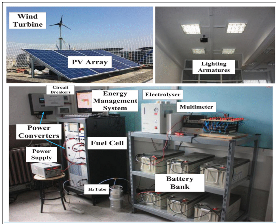
Figure 1.12 Experimental Set Up of Laboratory Scale of MG System
