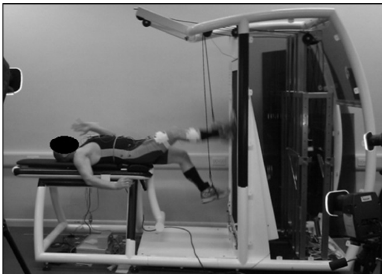
Figure 1.19 Tapis roulant vertical VertiRun (Sheffield, UK) Tirée de Jordan et al. (2017)
