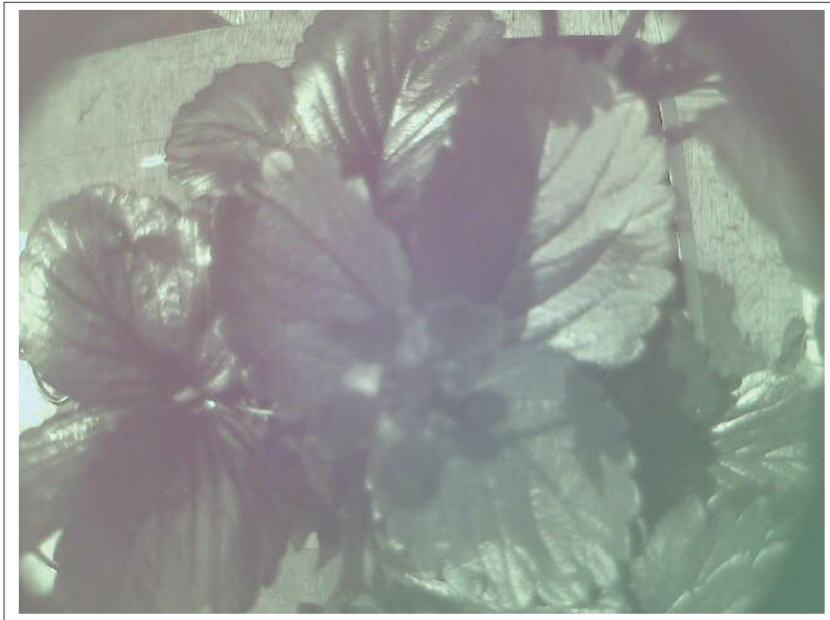
Figure 1.5 UV image of Strawberry cultivar using the NID with xNite BP1 and 330c external filters.
