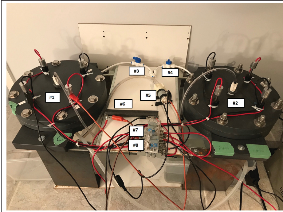
Figure 3.1 Testing bench: (#1):MCDI#1 cell, (#2):MCDI#2 cell, (#3):MCDI#1 feeding valve, (#4):MCDI#2 feeding valve, (#5):Main peristaltic pump, (#6):R_SC resistor (1 ohms), (#7):Relay switch SW1, (#8):Relay switch SW2
