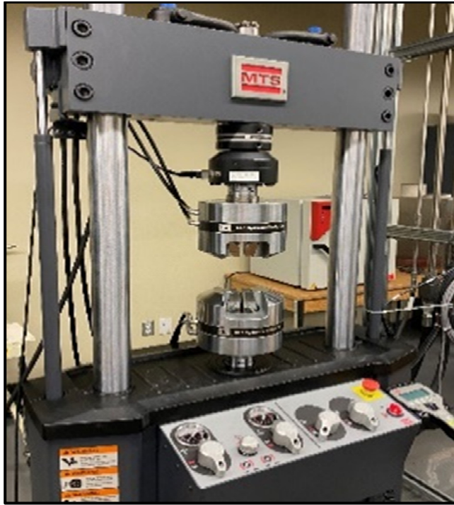
Figure 2.1 Hydraulic tensile compression machine used for the die expansion tests
