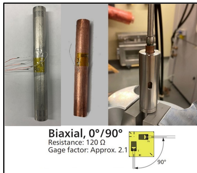
Figure 4.9 Expansion test workbench with SS316L and C122 3/8 in. tube samples and biaxial strain gage
