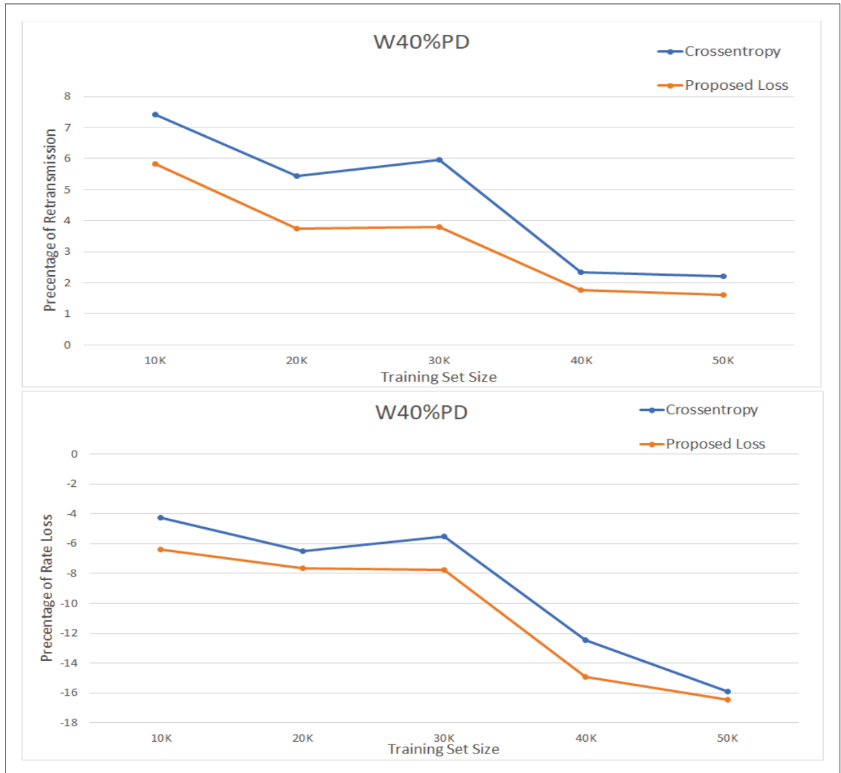
Figure 6.4 The percentage of retransmissions and rate loss for W40%PD in scenario C2 for models trained with crossentropy and our proposed loss function (6.6)
